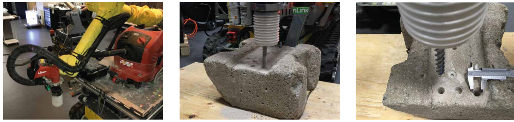
FIG. 4 Drilling test. Left: Serial arm robot UR10 mounted hosting a driller with integrated dust suctioning system. Centre: Drilling with a 16 mm drill bit into sample concrete. Right: Showing the quality of a drilled hole.
