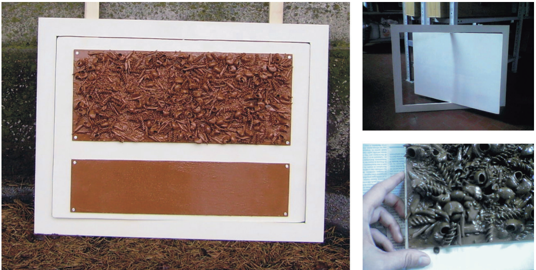
Fig. 2. Rotating target. The irregular surface of the upper module mounted on the white panel has a 1-cm mean length.
