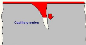
Figure 5. Penetrant capillary process ( http://Simula.com/ndtpt )
