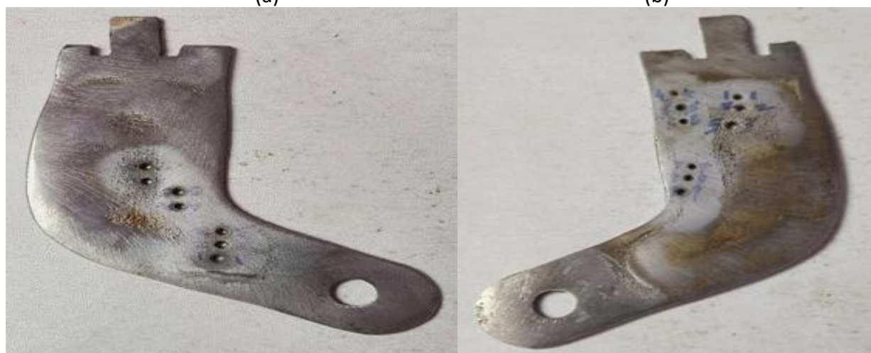
Figure 2. Machined EOS stainless steel 316L with (a) 7 holes and (b) 9 holes
