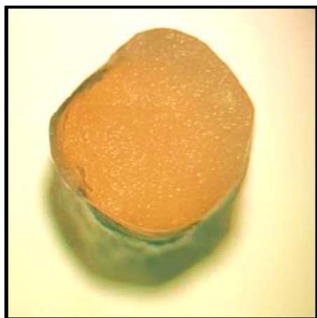
Figure 2- Stereo-microscopic picture at 80x magnification showing cohesive fracture in Group B
