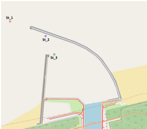
Figure 3 - Location of ADCP devices (St_1, St_2 and St_3) in the area of newly constructed Przekop Mierzei port, Poland.
