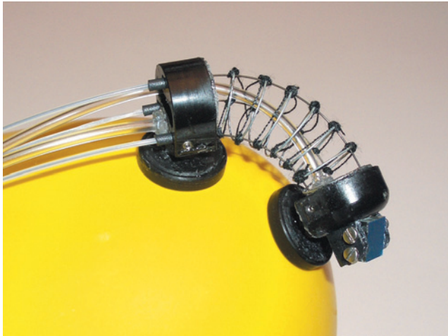
Figure 2. The HeartLander device is steered by advancing the 3 manipulator wires unequal amounts. With 3 wires spaced in a radially symmetric pattern, the device can steer not only left and right but also up and down. This method facilitates locomotion across the curved epicardium. The spring between the 2 solid modules prevents the drive wires from bowing outward during turns.
