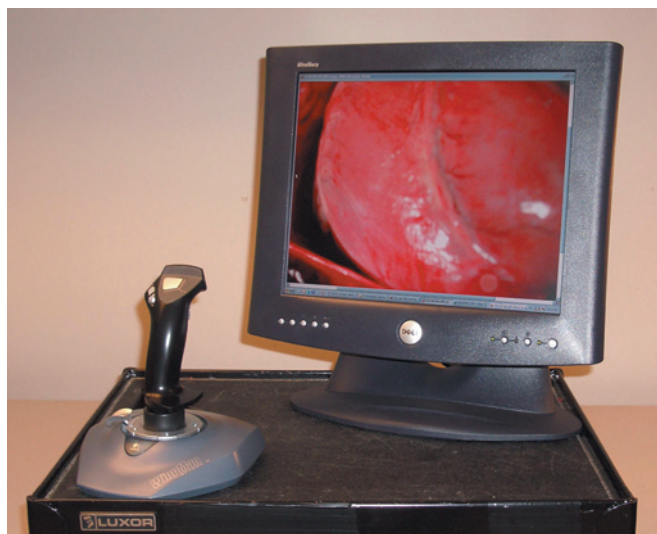
Figure 3. The HeartLander control interface. The joystick is used for control of locomotion, and the monitor is used to display video from the device camera.
