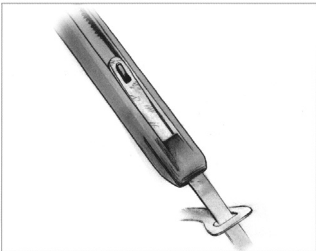
Figure 2. The narrow end of the steel band is inserted into the tensing device and connected through an eyelet to the hook of the set screw.
