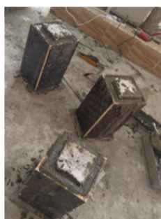
Fig. 6. Casting a square column with repaired material.
