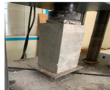
Fig. 7. Testing of concrete column damage after using the repaired material.
