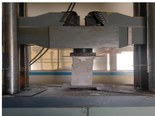
Fig. 5. Testing of concrete columns until 90% load compression damage.
