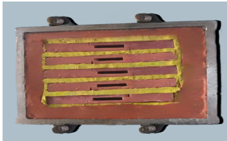
Figure 3. Specialized flask for packing the soft liner into the gaps between acrylic specimens.
