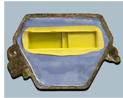
Figure 1. Silicone mold space inside dental stone after removing the plastic pattern.
